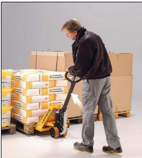
Travel direction is selected by an adjusting handgrip on the handle. Squeeze the handgrip, pump the handle and the truck will be powered in the walking direction. When the handgrip is pressed downward, and the handle is raised, the truck will be powered in the direction of the forks.
